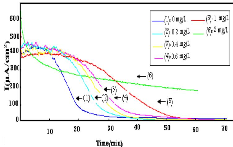
Figure 4. Chronoamperometric curves of Fourchi for an addition of the different concentrations of  $K_3PO_4$  at 20°C.
