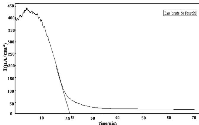
Figure 2. Chronoamperometric curve of Fourchi raw water at 20°C.
