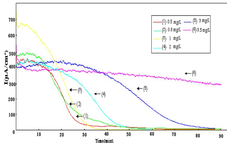
**Figure 5.** Chronoamperometric curves of Fourchi for an addition the different concentrations of  $K_2HPO_4$  at 20°C.
