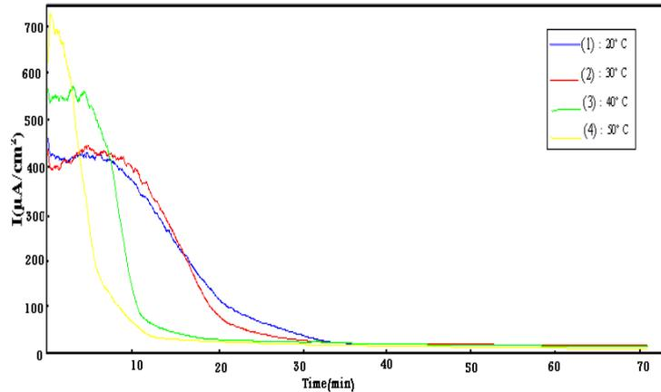
Figure 3. Chronoamperometric curves of raw water of Fourchi with different temperatures.
